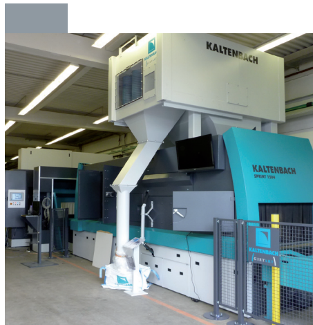
Shot blast and painting unit
